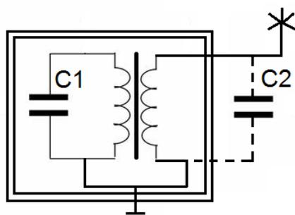
Fig. 2 Equivalent circuit diagram of the experimental setup, where C1 corresponds to the capacity of the electronic circuit of the GDV device, C2 - the equivalent capacitance of the antenna in the premises.
