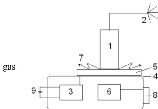
Fig. 1 The experimental setup. 1 - metal cylinder; 2 Antenna "GDV Sputnik"; 3 - high-voltage pulse generator; transparent conductive coating; 5 - transparent quartz electrode; 6 - video converter; 7 - discharge; 8 - USB-drive; 9 - Power Supply
